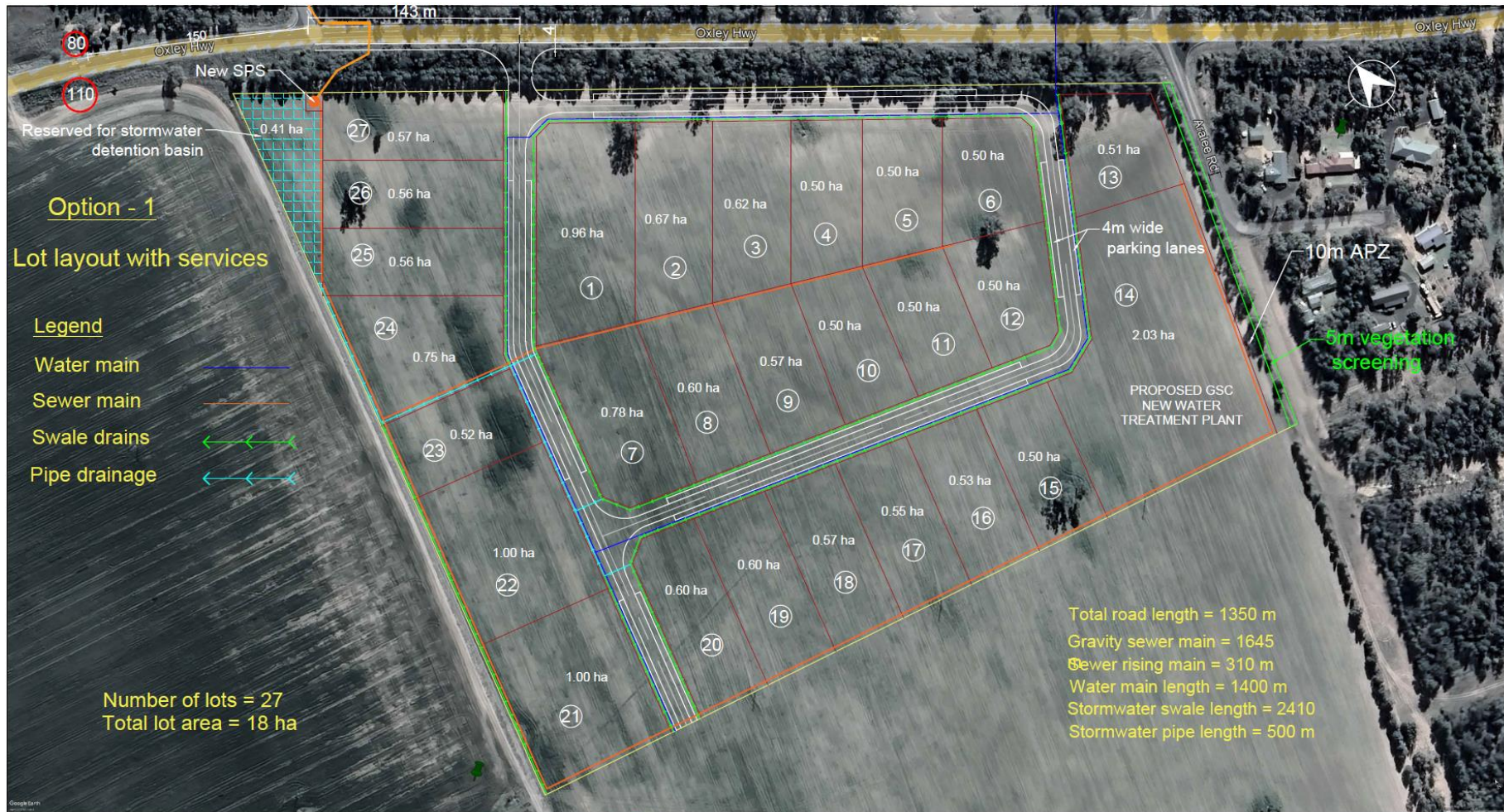
Figure 7: Indicative Site Layout – Northern Section (Industrial Area)
